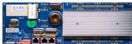
RS485 Communication between battery and inverter Band rate 9600bps RS485 Interface Communication between parallel packs or BMS and PC Band rate 9600bps
