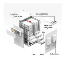
LiFePO4 cells + battery management system (BMS) + ...
