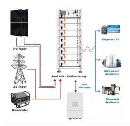
Systems (BESS) are based on lithium-ion batteries, offering advantages such as high energy ...
