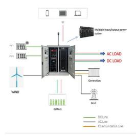
controller series, PV and wind system controller series, solar inverter.
